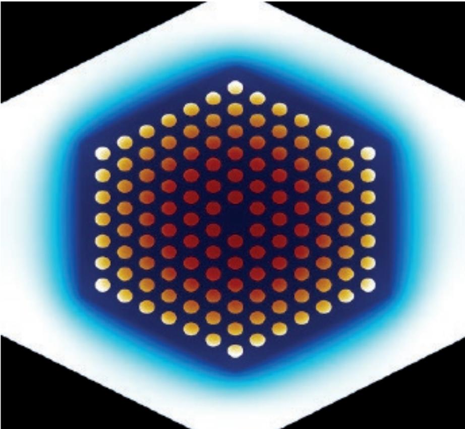
Graphics from the Serpent criticality safety calculation showing relative fission power (red-yellow colors) and thermal neutron flux (blue colors) in a VVER-440 fuel assembly.
