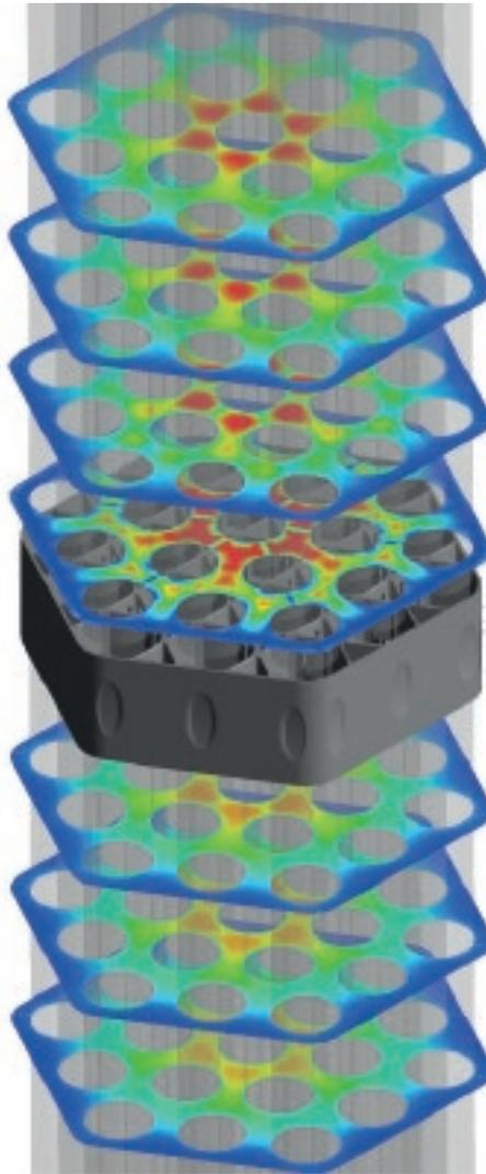
CFD-analysis showing the distribution of steam in cross sections around the upper spacer of a test assembly.
